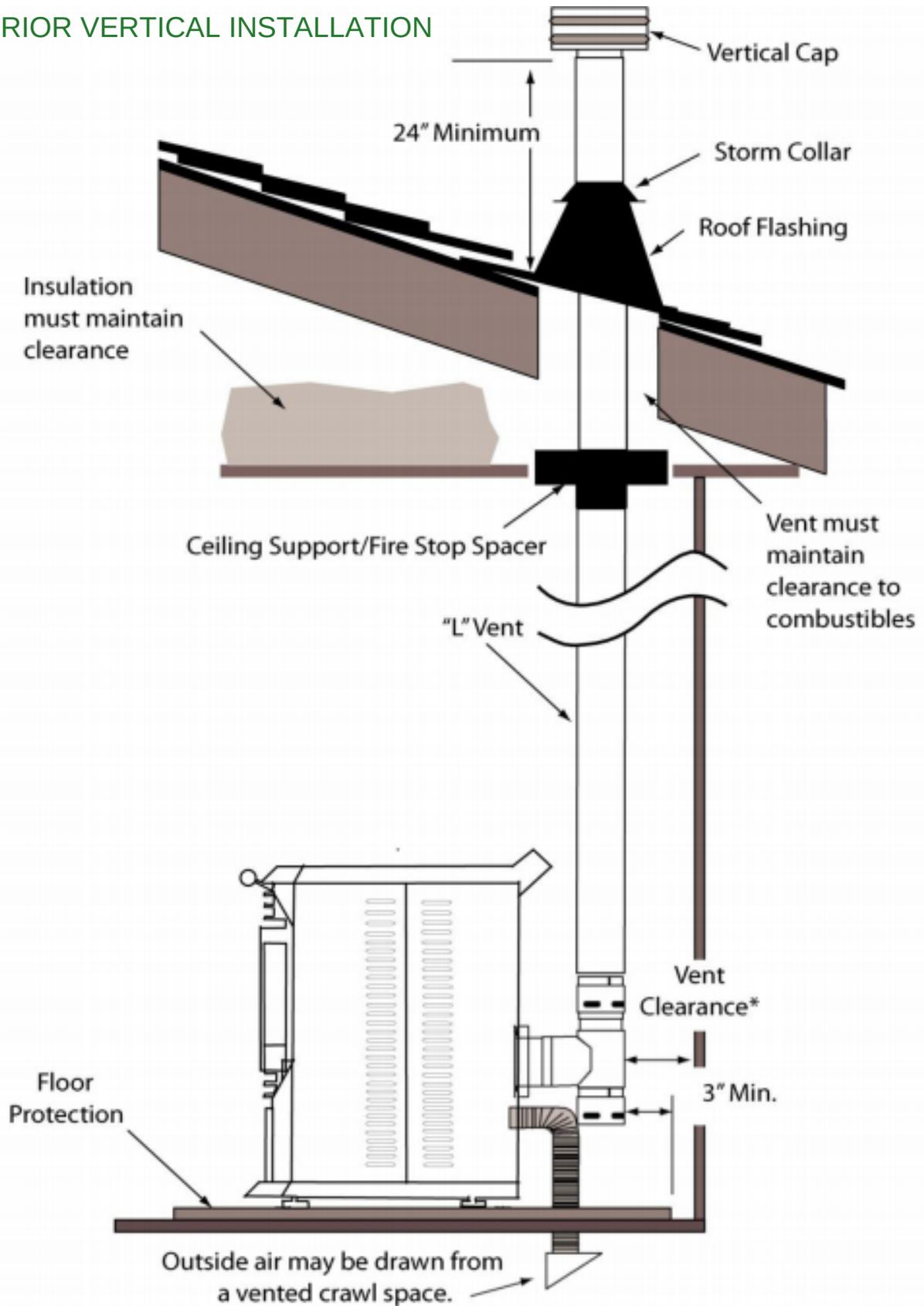
\* Install a vent at clearance specified by the vent manufacturer
