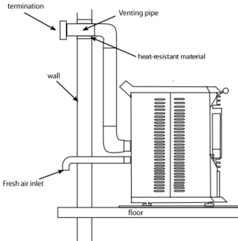
Figure 11: Straight Installation—inside vertical rise, horizontal termination
