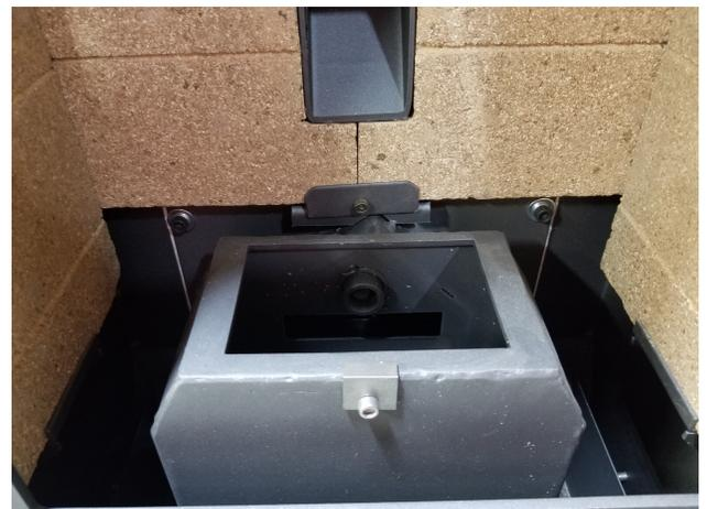
Figure 24: Burn Pot Cradle/Igniter Tube
