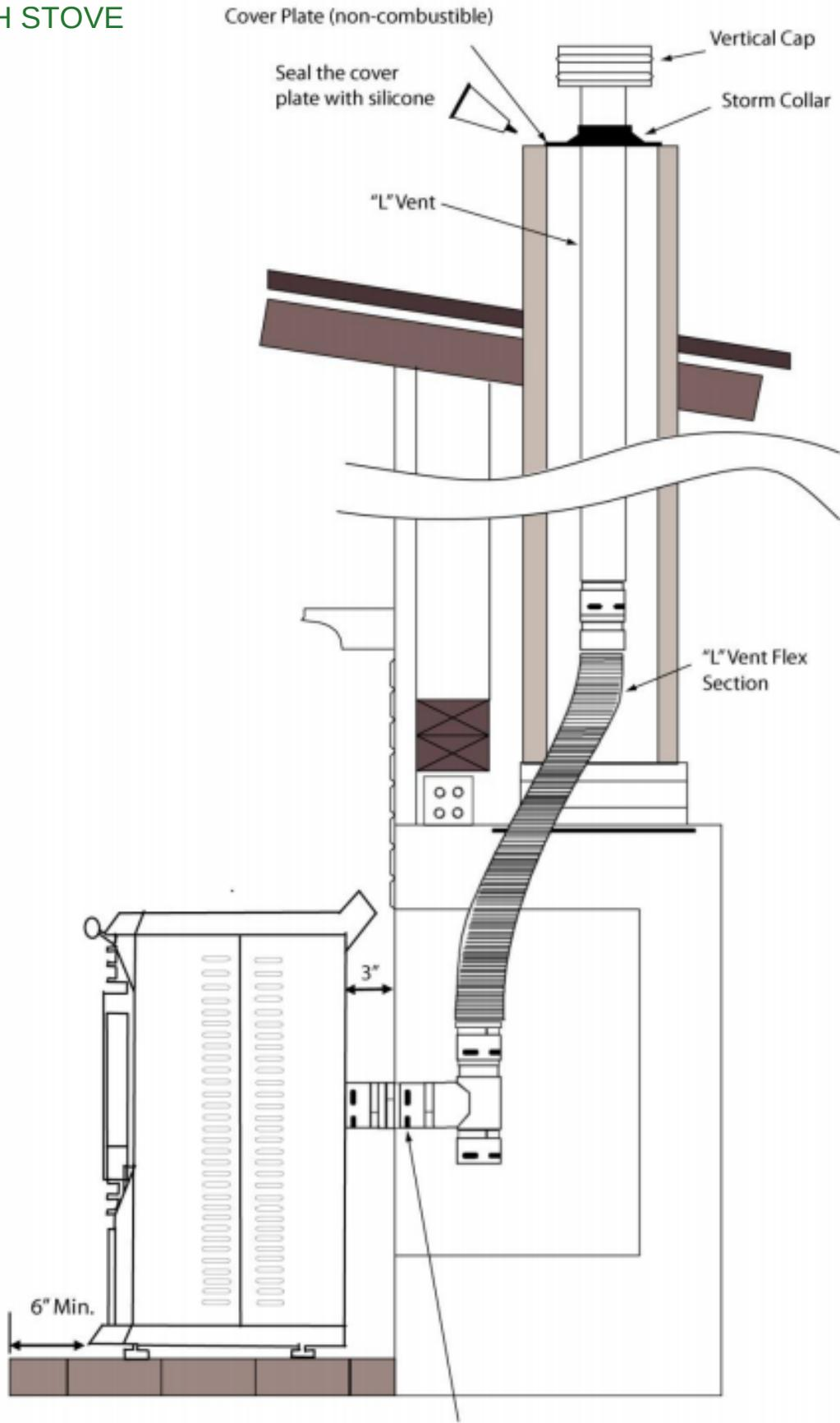
NOTE: you will probably need a short horizontal section here to clear the lintel and allow the hopper lid to open.
