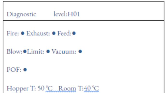
**Level:** Changing the level will allow you to test the component in the various heating power levels.
