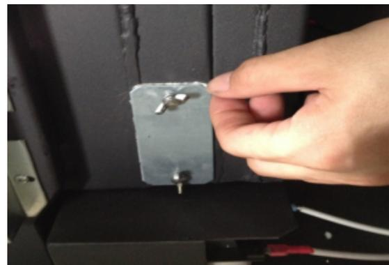
Figure 26: Exhaust Chamber Cover Plate.
