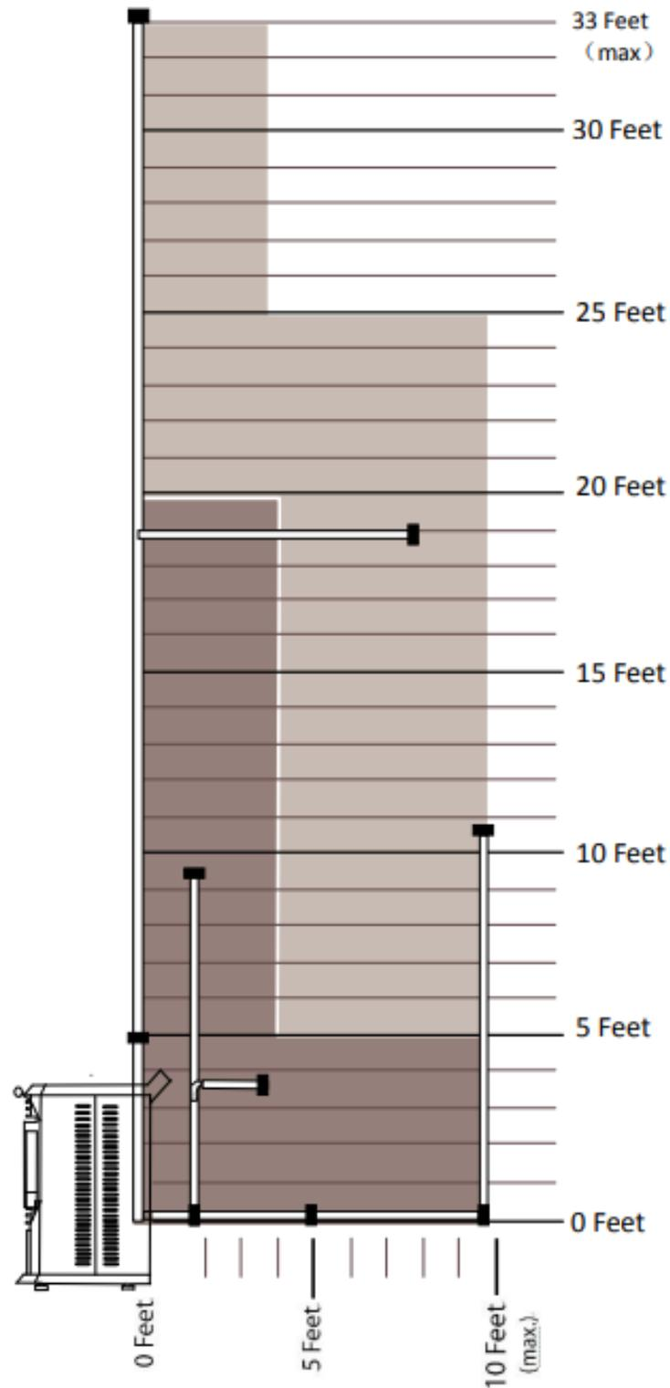
Figure 9: Venting and combustion motor voltage adjustment chart
