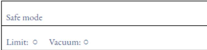
In the safe mode, you will have the ability to bypass these two components (Limit and Vacuum) of your stove to see if they are properly working.
