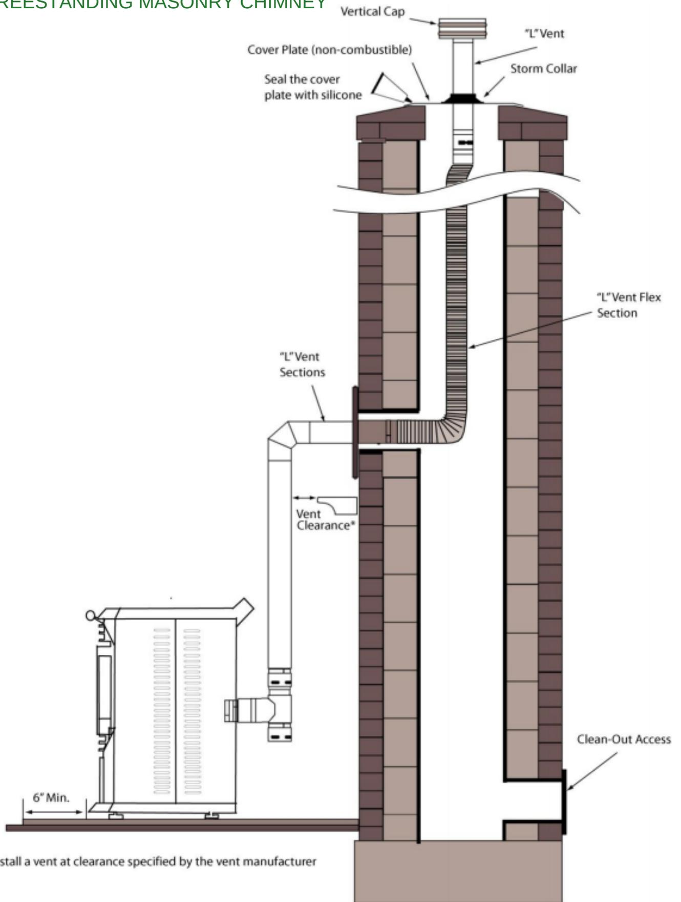
\* Install a vent at clearance specified by the vent manufacturer
