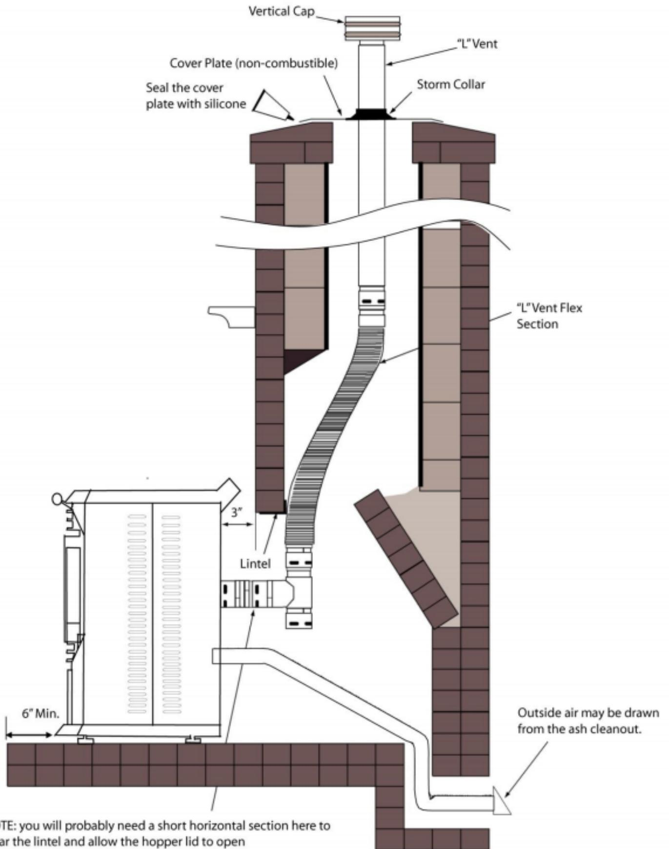
NOTE: you will probably need a short horizontal section here to clear the lintel and allow the hopper lid to open
